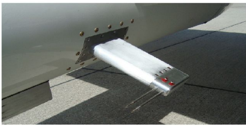
Fig.6. Two UFT-II thermometers with housing designed and built by Enviscope in course of DENCHAR field intercomparison campaign.
