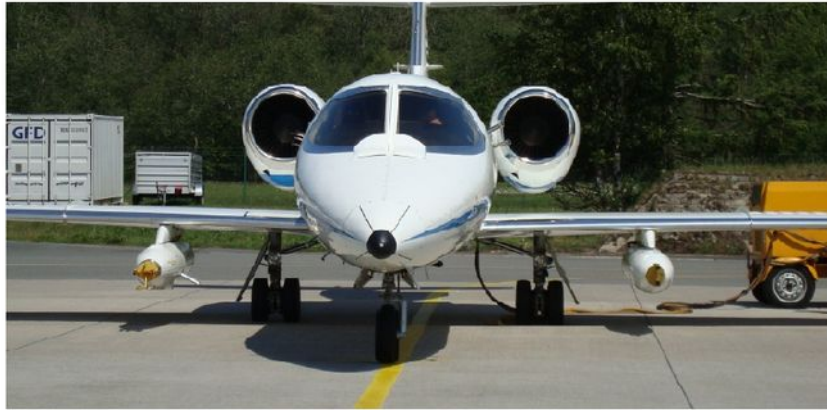
Fig.7. UFT-2 in housing attached to the container under the left wing of Learjet aircraft.
